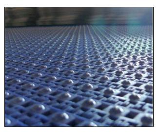
The SigSorter table ejects the bundle onto a customer supplied conveyor. The close-up view of the powered ball table showing the close spacing of the driven table balls for optimised bundle rotation, handling and movement. The unit ensures minimum product contact and maximum product protection for zero-defect bundle delivery, even on the smallest and most sensitive products such as RRP cases.
