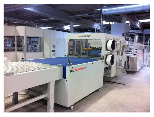
Located behind the ISB Inline Bundle squaring and strapping machine the zero defect bundle ejection table is controlled by the ISB PLC Unit. Any defective bundles identified by the upstream FFG units glue control or print quality-check camera are automatically removed, after strapping, by the ejection table. This ensures that any incorrectly glued or printed bundles do not pass to the palletising area aiding the objective of zero-defect product delivery to end-users.
