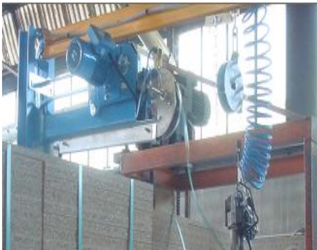
PSF loop for auto strap re-feed to reduce operator effort model with VT pneumatic hand tool for PET Tenax® Polyester heavy duty strapping
