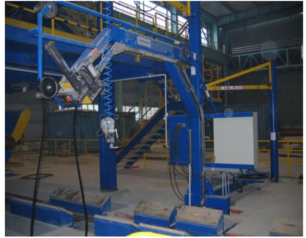
Simple overview showing PSF to strap coils around, the circumference in a heavy-duty metals industry application
