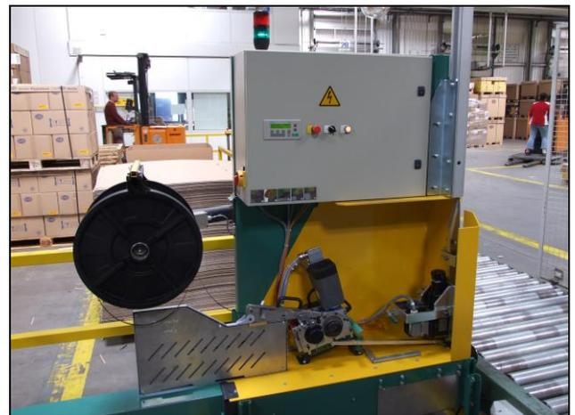
Set up of the Feeder and Sealer Modules with easy machine operator access and operations and for service work.
