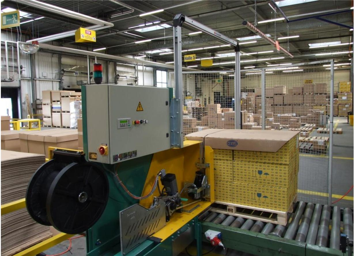
MH-VRB Side-Seal Machine shown in a high through-put production plant strapping palletised and packaged automotive components ready for shipment worldwide
