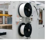
Automatic coil splicing Strap is automatically spliced from a second dispenser to provide up to 20,000m of strap for continuous production with zero downtime.
