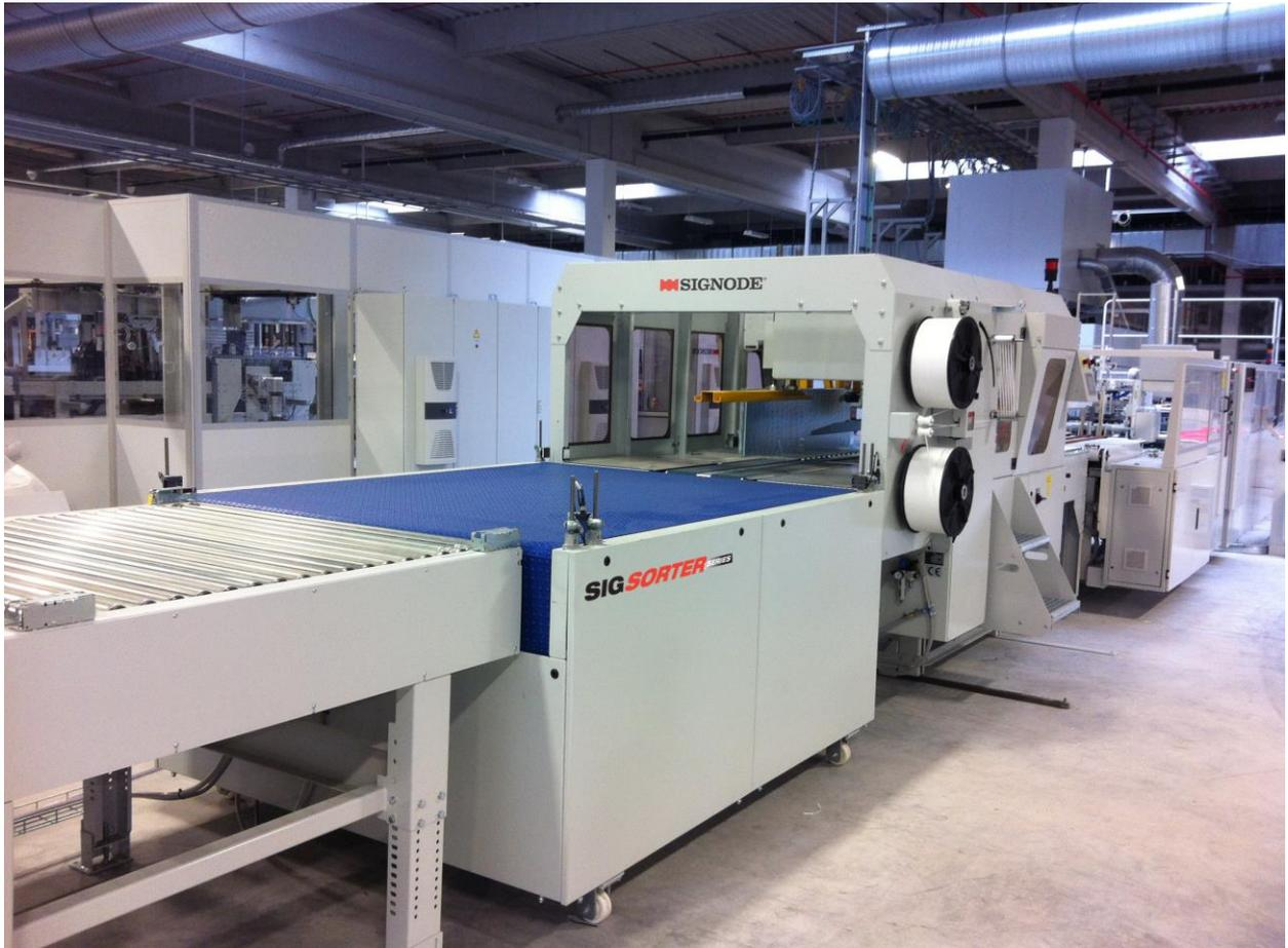
Located behind the ISB Inline Bundle squaring and strapping machine the zero defect bundle ejection table is controlled by the ISB PLC Unit. Any defective bundles identified by the upstream FFG units glue control or print quality-check camera are automatically removed, after strapping, by the ejection table. This ensures that any incorrectly glued or printed bundles do not pass to the palletising area aiding the objective of zero-defect product delivery to end-users.
