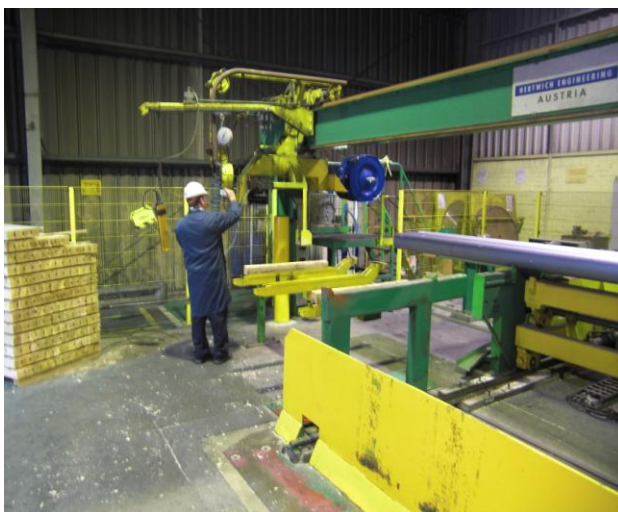
PSF loop for auto strap re-feed to reduce operator Effort, model with a pneumatic hand tool for PET
