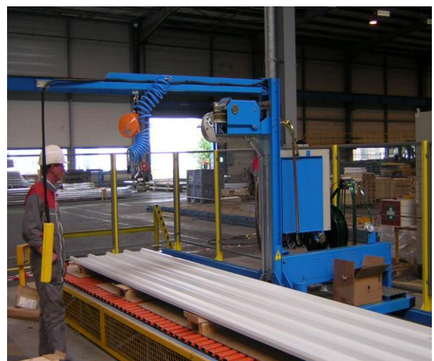
Simple overview showing PSF to strap sheet metal metal cladding products - moving version over 10m
